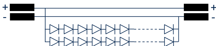
LED on-board circuit
